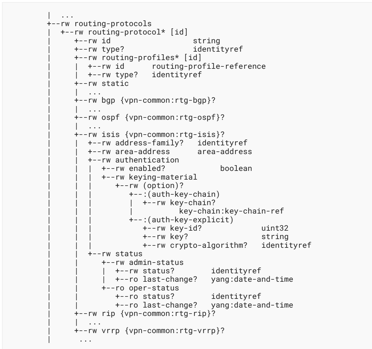
Figure 18: IS-IS Tree Structure
