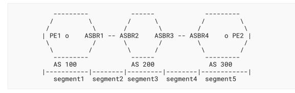
The inter-AS segmentation procedures specified so far ([RFC6513], [RFC6514], [RFC7117], and Section 5 of this document) require all ASBRs to be involved, and ingress replication is used between two ASBRs in different ASes.
